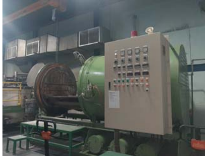
Vacuum pyrolysis machine
